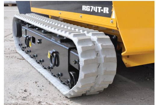
Rubber track undercarriage retracts to fit through 36" gates
