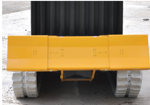
The wide hydraulic backfill blade saves time during clean up.
