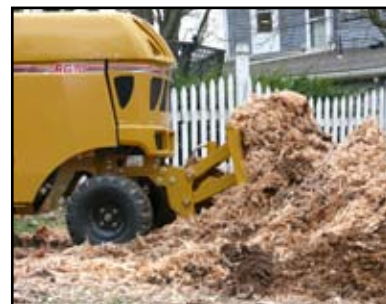
Hydraulic Backfill Blade
