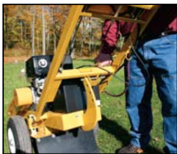
Adjustable handlebars to accommodate operators of all sizes
