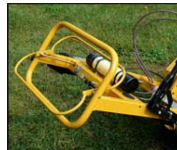
All models feature operator presence safety bar
