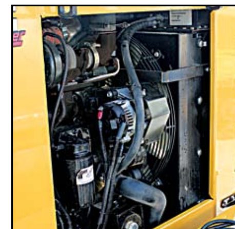
Cummins diesel engines in 130 hp or 160 hp
