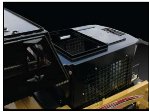
Roof Top Escape Hatch
