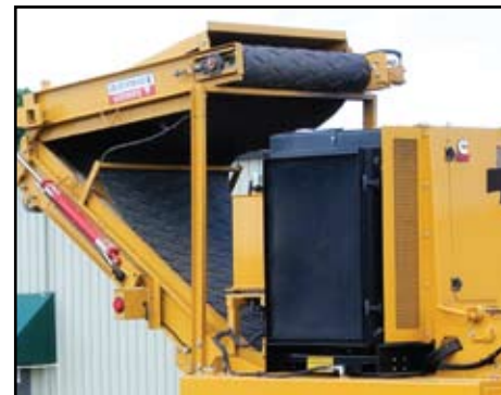
Folding Extended Discharge Conveyor with Magnetic Head Pulley
