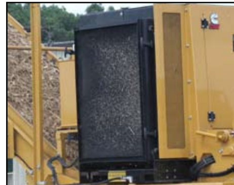
Oversized Radiator with Reversing Fan and Removable Debris Screen
