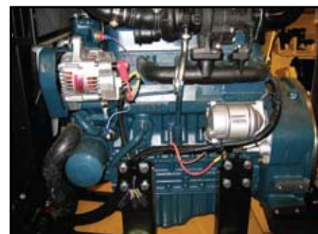
44 hp Kubota Engine Meets Tier IV Emissions
