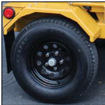
13" Wheel and Torflex® suspension axle
